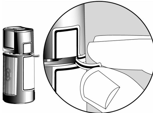
5. To open the bottle, unscrew the cap by turning as indicated by the arrows on the top of the cap. Do not pull the cap directly up and away from the bottle. Pulling the cap directly up will prevent your dispenser from operating properly.
